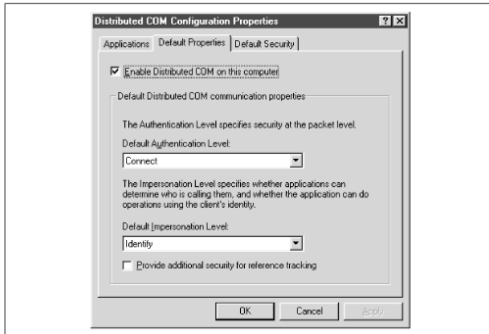
Figure 12-5.DCOM configuration tool with DCOM enabled
