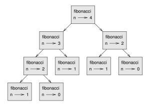
A call graph shows a set function frames, with lines connecting each frame to the frames of the functions it calls. At the top of the graph, fibonacci with n=4 calls fibonacci with n=3 and n=2. In turn, fibonacci with n=3 calls fibonacci with n=2 and n=1. And so on.
