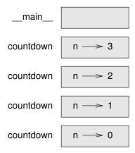
As usual, the top of the stack is the frame for \_\_main\_\_. It is empty because we did not create any variables in \_\_main\_\_ or pass any parameters to it.
