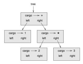
The nodes of an expression tree can be operands like 1 and 2 or operators like + and \*. Operands are leaf nodes; operator nodes contain references to their operands. (All of these operators are **binary**, meaning they have exactly two operands.)
