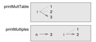
The value of i in printMultTable goes from 1 to 6. In the diagram it happens to be 3. The next time through the loop it will be 4. Each time through the loop, printMultTable calls printMultiples with the current value of i as an argument. That value gets assigned to the parameter n.
