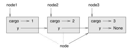
By convention, lists are often printed in brackets with commas between the elements, as in [1, 2, 3]. As an exercise, modify printList so that it generates output in this format.
