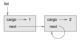
If we invoke printList on this list, it will loop forever. If we invoke printBackward, it will recurse infinitely. This sort of behavior makes infinite lists difficult to work with.
