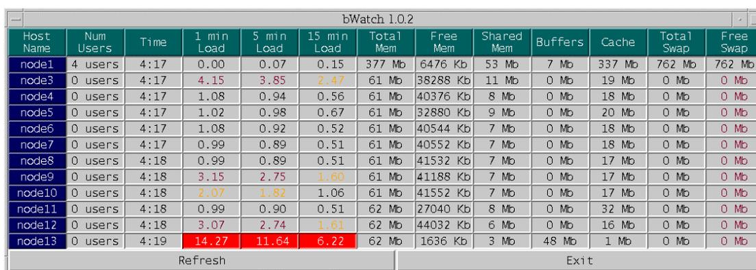
The screenshot shows the bWatch 1.0.2 application window. It contains a table with 13 columns: Host Name, Num Users, Time, 1 min Load, 5 min Load, 15 min Load, Total Mem, Free Mem, Shared Mem, Buffers, Cache, Total Swap, and Free Swap. The table lists data for nodes node1 through node13. Node 13 has the highest load, with 14.27 at 1 min, 11.64 at 5 min, and 6.22 at 15 min. The interface also includes 'Refresh' and 'Exit' buttons at the bottom.
