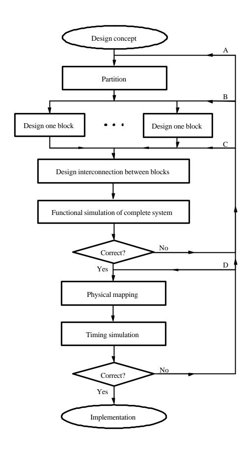
Figure 1.6 Design flow for logic circuits
