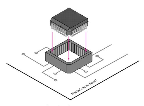
Figure 3.31 A PLCC package with socket.
