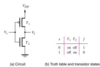
Figure 3.12 CMOS realization of a NOT gate.
