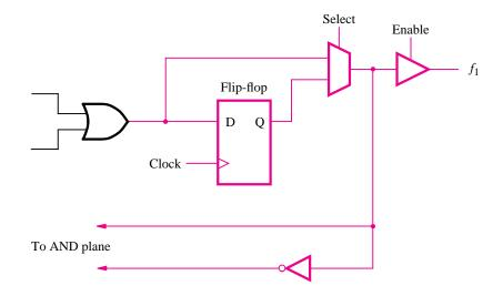
Figure 3.29 Extra circuitry added to OR-gate outputs from Figure 3.28.
