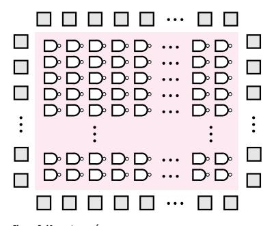
Figure 3.41 A sea-of-gates gate array.
