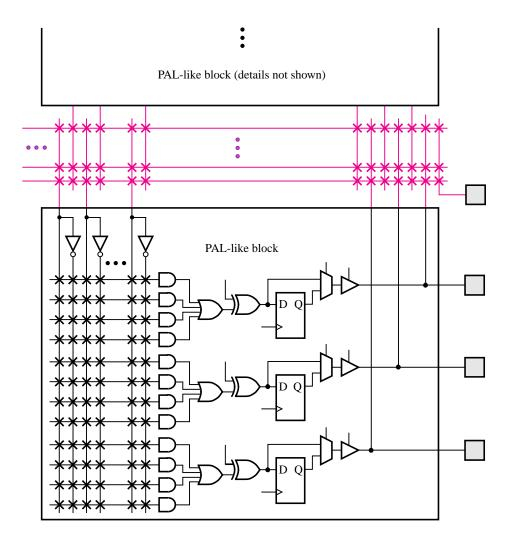
Figure 3.33 A section of the CPLD in Figure 3.32.
