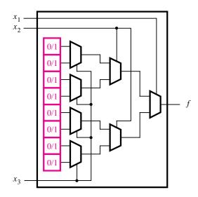
Figure 3.37 A three-input LUT.
