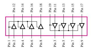
**Figure 3.23** The 74244 buffer chip.
