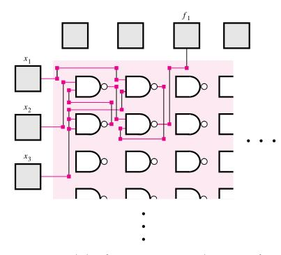
**Figure 3.42** The logic function  $f_1 = x_2 \overline{x}_3 + x_1 x_3$  in the gate array of Figure 3.41.
