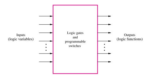
Figure 3.24 Programmable logic device as a black box.
