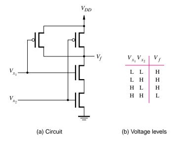
Figure 3.18 Voltage levels in the circuit in Figure 3.13.
