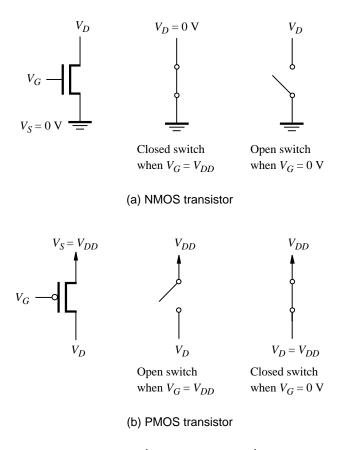
NMOS and PMOS transistors in logic circuits. Figure 3.4
