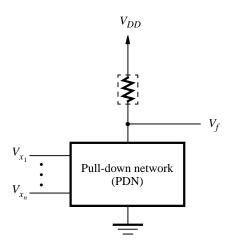
Figure 3.10 Structure of an NMOS circuit.
