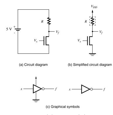
Figure 3.5 A NOT gate built using NMOS technology.
