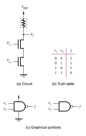
Figure 3.6 NMOS realization of a NAND gate.
