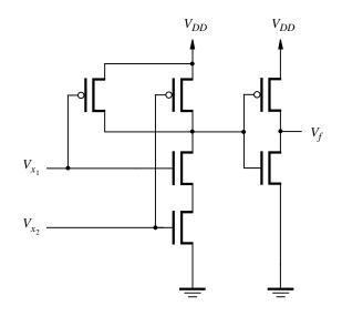
Figure 3.15 CMOS realization of an AND gate.
