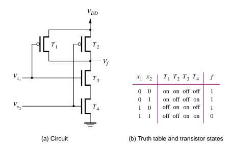
Figure 3.13 CMOS realization of a NAND gate.
