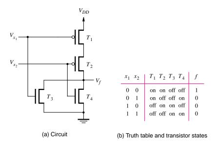
Figure 3.14 CMOS realization of a NOR gate.
