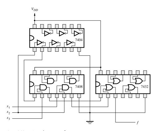
**Figure 3.22** An implementation of  $f = x_1x_2 + \overline{x}_2x_3$ .
