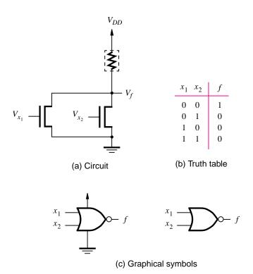
Figure 3.7 NMOS realization of a NOR gate.
