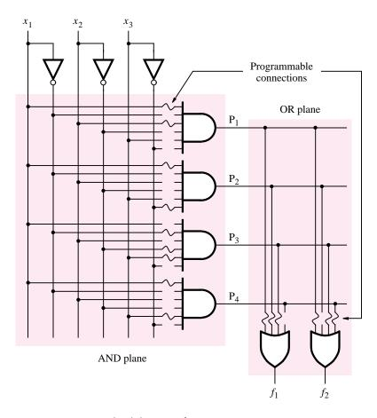
Figure 3.26 Gate-level diagram of a PLA.
