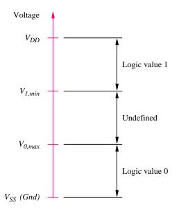
Figure 3.1 Representation of logic values by voltage levels.
