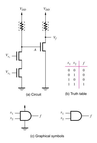
Figure 3.8 NMOS realization of an AND gate.
