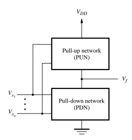
Figure 3.11 Structure of a CMOS circuit.
