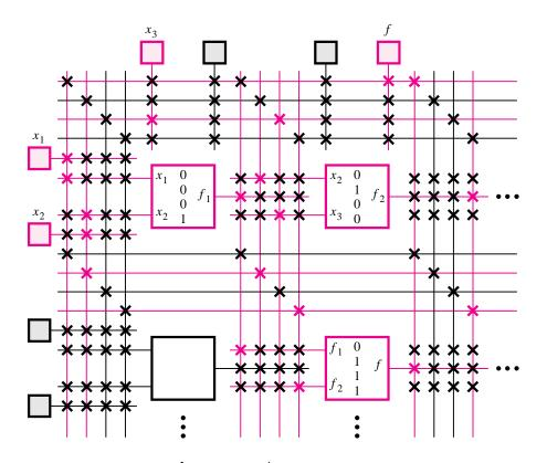
Figure 3.39 A section of a programmed FPGA.
