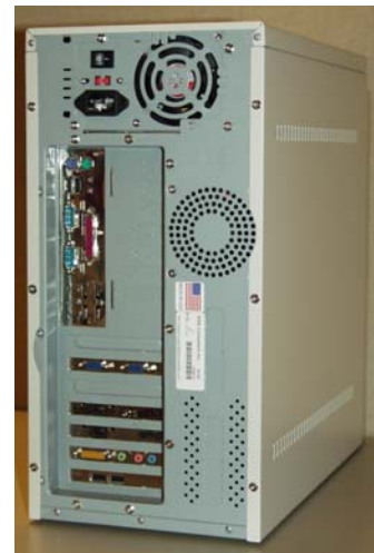
Figure 1.3. Ports on a PC. The serial ports and Ethernet interface cards are labeled.
