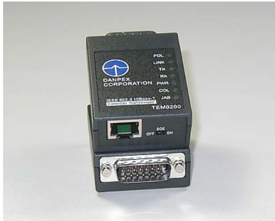
Figure 1.10. Two AUI/RJ-45 transceivers – the top one shows the RJ-45 end, the bottom one shows the AUI end.
