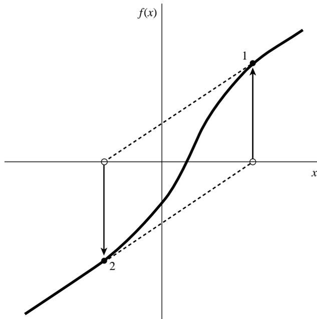
Figure 9.4.3. Unfortunate case where Newton's method enters a nonconvergent cycle. This behavior is often encountered when the function  $f$  is obtained, in whole or in part, by table interpolation. With a better initial guess, the method would have succeeded.
